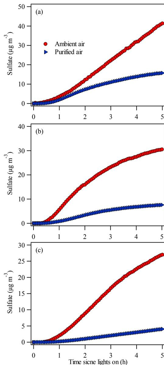
**Fig. 7.** Concentration of wall loss corrected sulfate derived from AMS data in ambient air experiment (red) and purified air experiment (blue) during 5 h of irradiation. (a) low NO condition (80 ppbv NO, Expt. 1 and 5), (b) high NO condition (200 ppbv NO, Expt. 2 and 6), (c) low  $NO_2$  (80 ppbv  $NO_2$ , Expt. 3 and 7). (For interpretation of the references to colour in this figure legend, the reader is referred to the web version of this article.)
