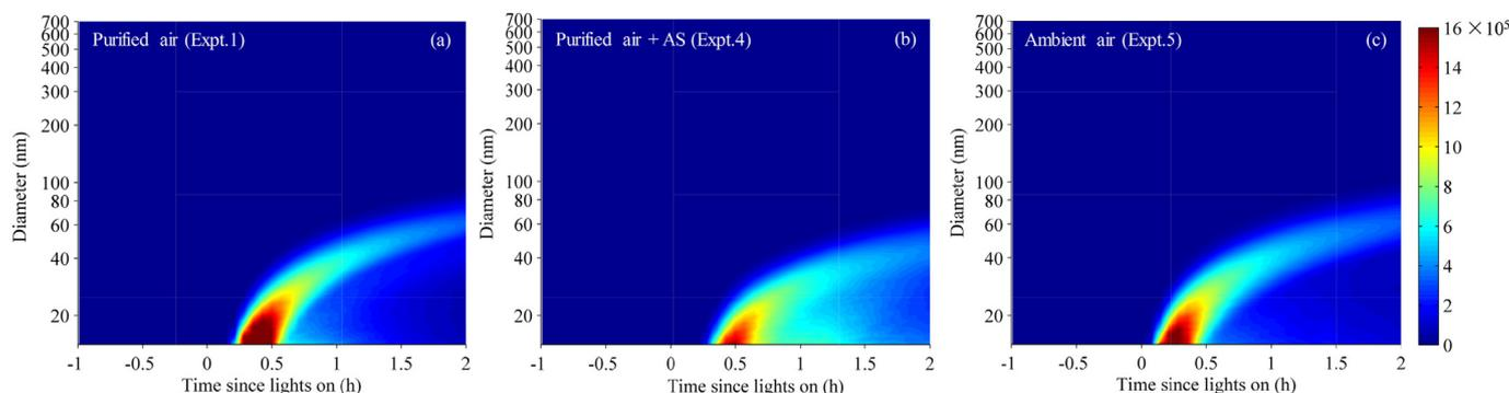
**Fig. 3.** Particle size-number distributions for (a) purified air experiment without  $(\text{NH}_4)_2\text{SO}_4$  (Exp.1), (b) purified air experiment with  $(\text{NH}_4)_2\text{SO}_4$  (Exp.4) and (c) ambient air experiment (Exp.5).
