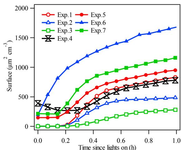
**Fig. 4.** Evolutions of surface areas for all experiments measured by SMPS in 1 h after lights were turned on. Line with open symbols represent purified air experiments, line with solid symbols represent ambient air experiments. Circle represents low NO condition (80 ppbv NO), triangle represents high NO condition (200 ppbv NO), square represents low  $\text{NO}_2$  condition (80 ppbv  $\text{NO}_2$ ).
