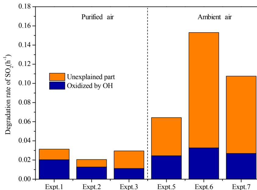
**Fig. 8.** The degradation rate of SO<sub>2</sub> during purified and ambient air experiments. The oxidation rate of SO<sub>2</sub> reacting with OH was calculated by the reaction rate coefficient and the average OH concentration.
